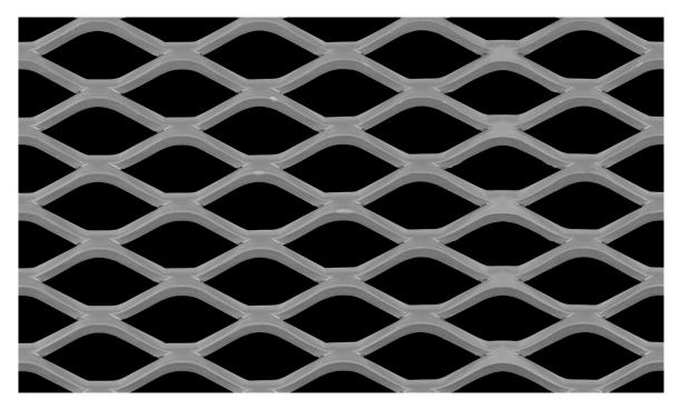
LW Pitch:38.10mmStrand Width:3.00mmSW Pitch:18.00mmThickness:3.00mmWeight:7.85 kg / m2Open Area:66%
